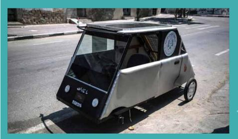
Palestine – Inspired by the permanent electricity blackouts and diesel shortage in the besieged Gaza Strip, two students from the Mechatronics Department, Faculty of Engineering and Information Technology at Al Azhar University-Gaza have built Gaza's first prototype solarpowered car, going for renewable, alternative and clean energy.
